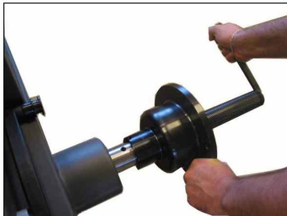
The adapter may differ in Air model (Pneumatic clamping)
